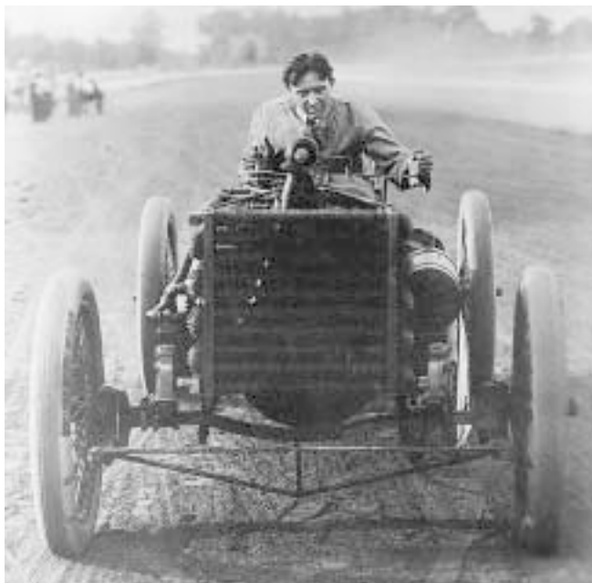
A head-on view of Oldfield and 999. Note the exposed valve train (with an overhead cam at this point) and the modified finned-tube radiator. AMATEUR ATHLETIC FOUNDATION OF LOS ANGELES
